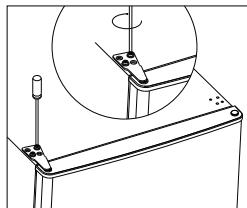
14. Clap in the hinge cover and hole cover on the top of unit.
