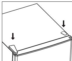
15. Check whether the door gasket is deformed. If yes, detach the fridge and the freezer door gaskets and then attach them after rotating.
