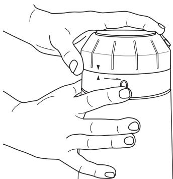
4. Keep the UNLOCK button pressed and lift the upper millstone by the grip with your other hand to remove it - see picture below. Release the button.
