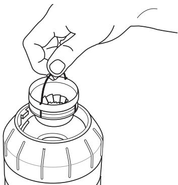
3. Press and hold the UNLOCK button at the back of the grinder base. Turn the milling fineness control knob anticlockwise with your other hand until the graphic mark on the milling fineness control is aligned with the one on the grinder base. This upper millstone can be only removed in this way - see figure below.
