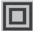
This equipment is protected by a double insulation.
