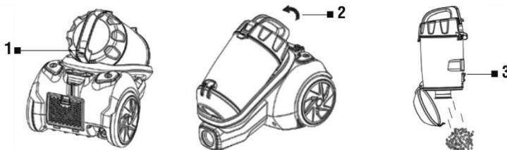
1. Release the dust tank by pressing the release button (1). Lift the hopper out of the vacuum cleaner body (2). Press the button to open it (3), the base of the hopper opens and the dust falls into the trash.
