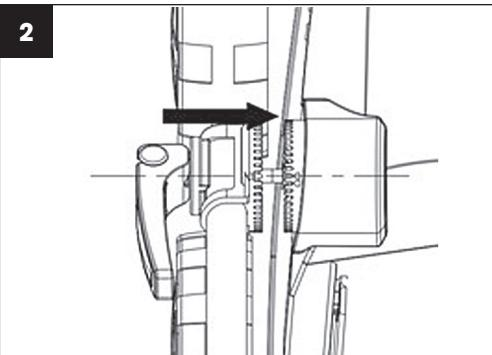
2. Screw on the handle's middle part with the power cord safety clamp attached using the fast coupling lever and the handle screw (fig. 3).
