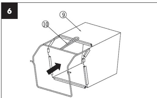
6. Installation of the completely assembled collection basket on to the scarifier (fig. 7).
