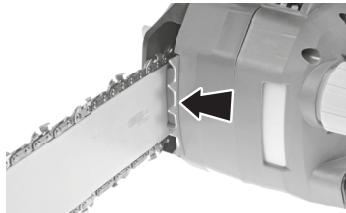
The claw stop enables the motor block to be secured to the wood when using pull saws. Uncontrolled kickback of the saw is thus made more difficult. The process also exerts pressure on the saw chain thanks to the generated leverage.
