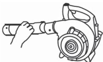
Put blow pipe B to the machine by rotating
