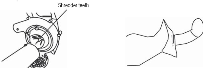
Open the fan cover, connect inhale pipe No.1 and No.2
