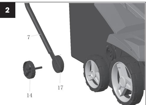
2. Screw on the handle's middle part with the power cord safety clamp attached using the fast coupling lever and the handle screw (fig. 3).
