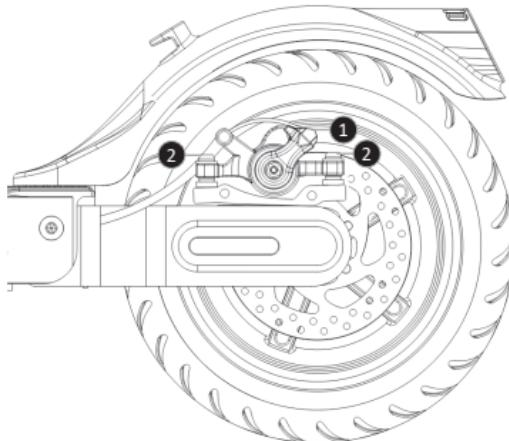
b) Removed brake caliper – rear view
