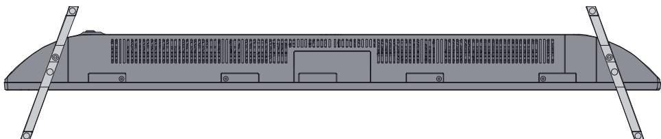
**English:** To assemble the base stand to the TV you will need a cross head screwdriver. To avoid damage to the TV screen during assembly ensure the TV is placed on a soft flat surface with the LCD screen facing downwards.
